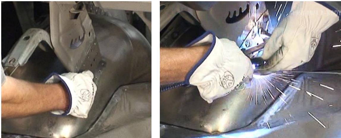
Figure 32 – Fabricate and Weld the Decklid Support
