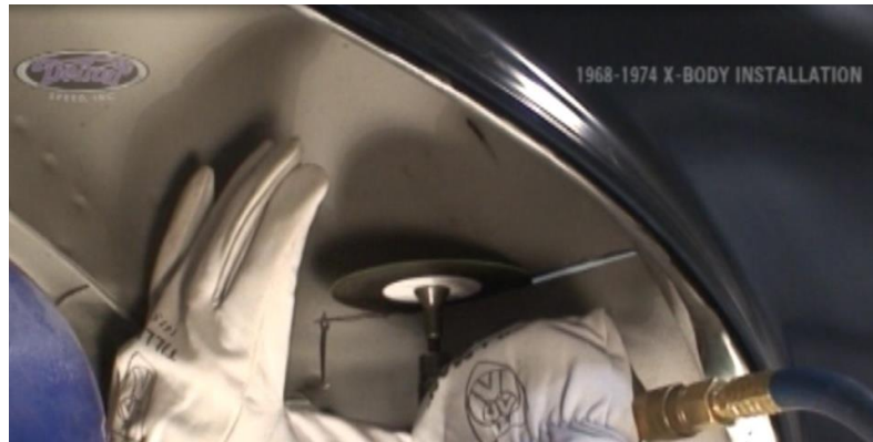
Figure 10 – Start Cutting the Stock Tub
