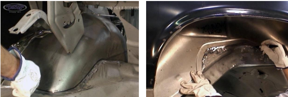
Figure 26 – Mark the Mini-Tub
