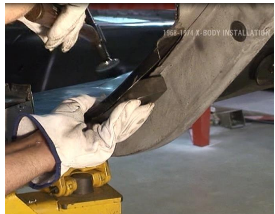
Figure 21 – Folding & Shaping of the Flange
