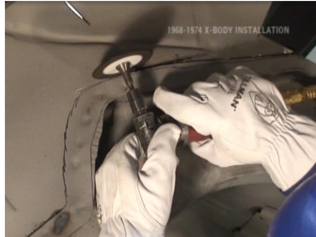
Figure 13 – Cut Pre-Marked Lines
