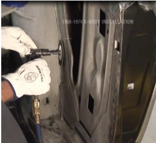
Figure 13 – Cut Pre-Marked Lines
