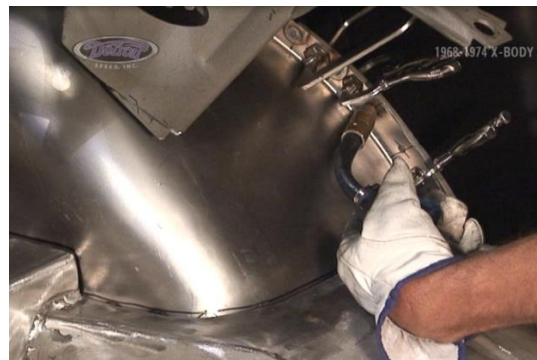
Figure 38 – Clamp and Weld to the Vehicle
