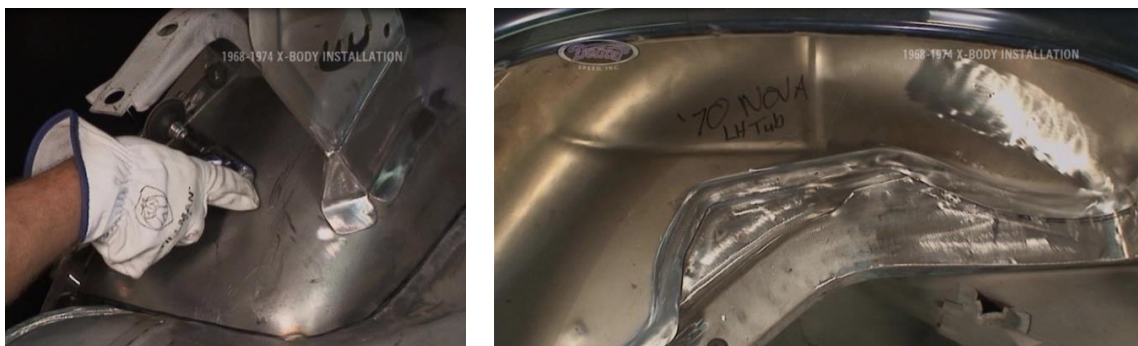
Figure 33 – Finish Grind Mini-Tub
