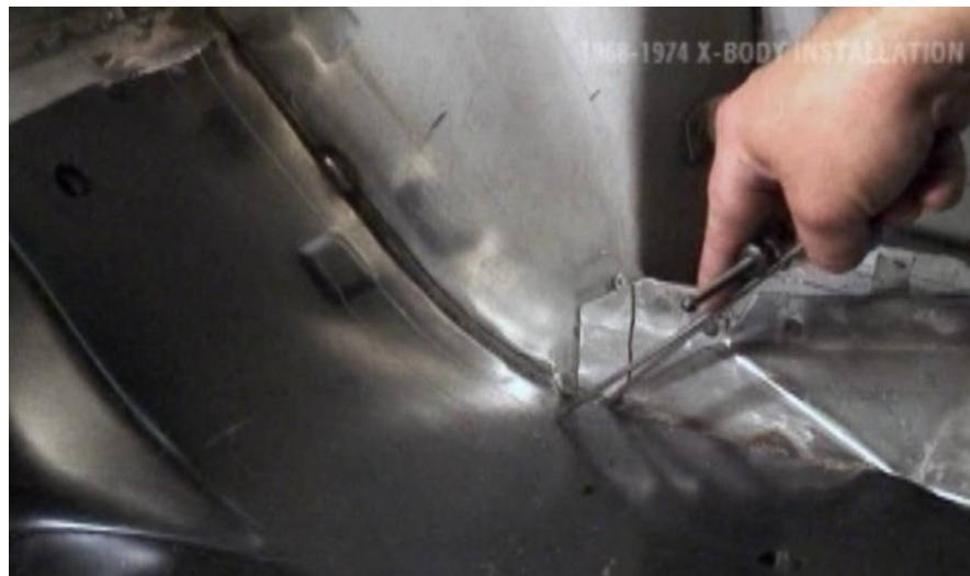
Figure 4 – Mark the Flange Bend Line
