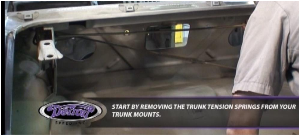
Figure 1 – Removing the Torsion Springs
