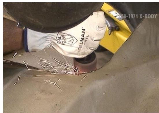
Figure 20 – Finish Cut and Grind Pre-Marked Lines
