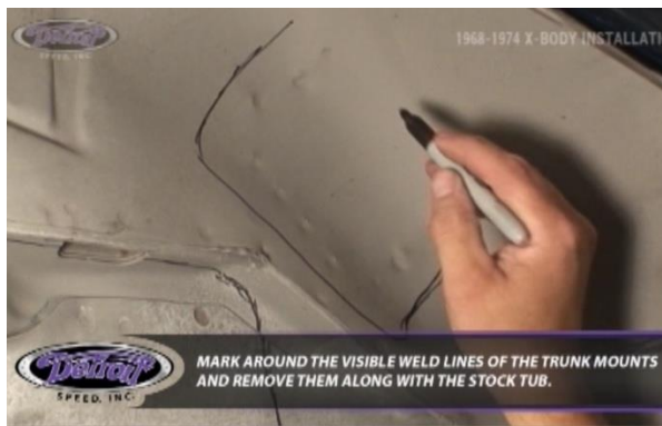
Figure 11 – Mark the Trunk Mounts
