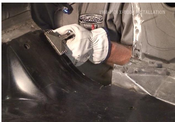
Figure 21 – Folding & Shaping of the Flange
