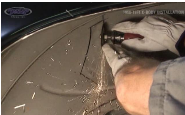
Figure 15 – Remove the Seat Brace
