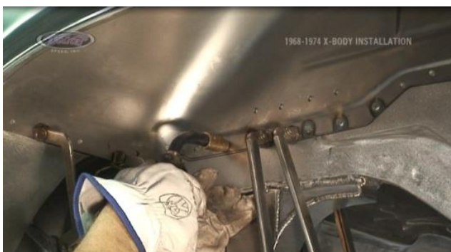
Figure 38 – Clamp and Weld to the Vehicle
