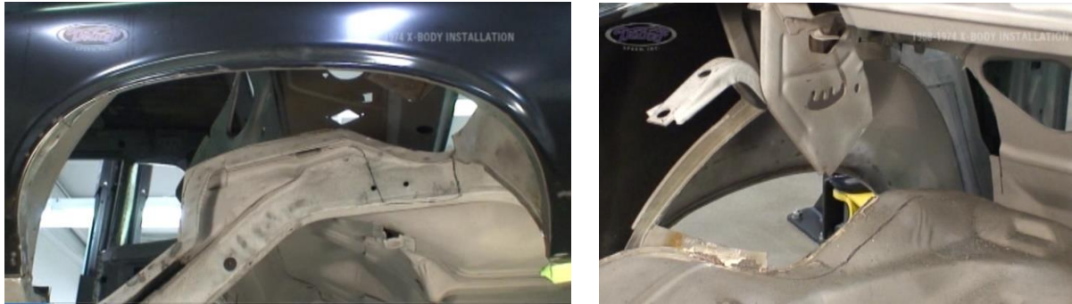
Figure 16 – Stock Inner Tub Removed
