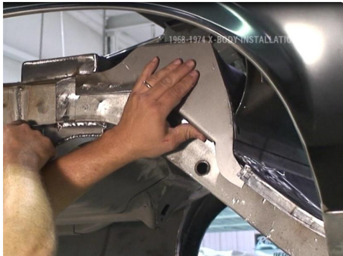
Figure 36 – Passenger Side Closeout
