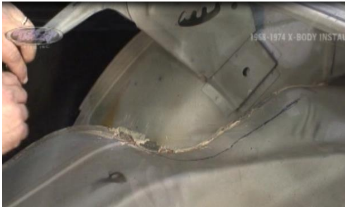
Figure 3 – Mark the Cut Lines
