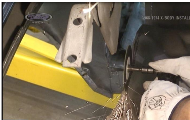
Figure 20 – Finish Cut and Grind Pre-Marked Lines
