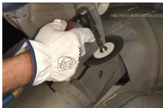
Figure 12 – Cut and Remove the Hinge Mount
