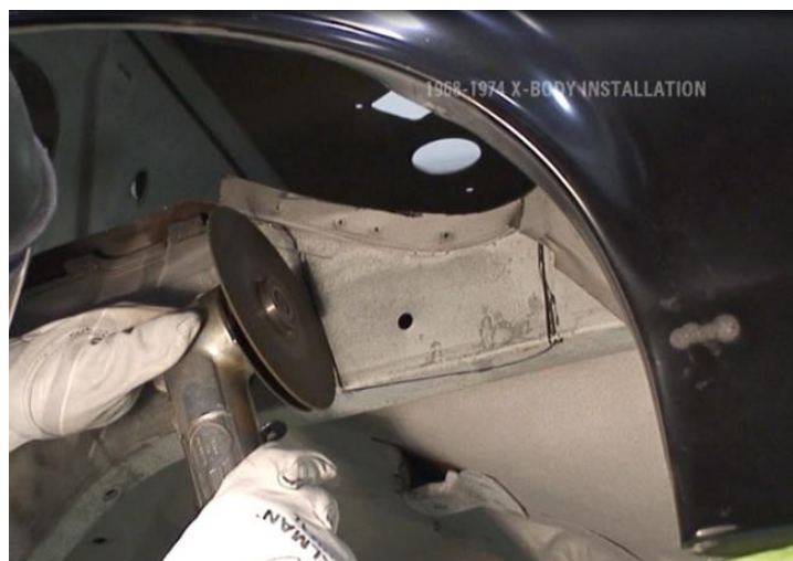
Figure 18 – Notch the Framerail
