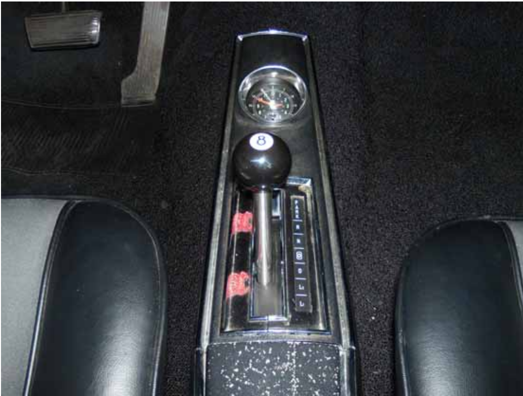
Shifter installed with 8 inch handle and Smoothie 8 Ball knob
