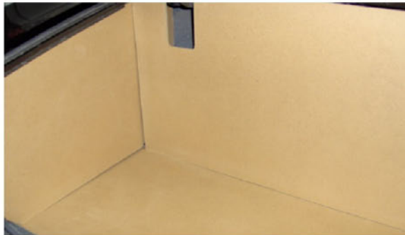
The next panel in is the back panel with the notchs for the hinges. Tilt the panel toward the back and then tilt into place under each hinge.
