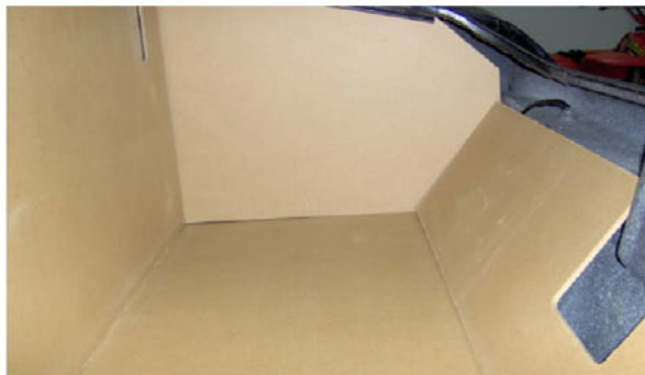
The last panel is the rear panel that fits under the trunk latch hold down. The panels may need to be sanded down if using thick material.
