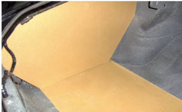
The left side is next and should be snug against the rear tail light housing area. The top of the panel should be inside the the trunk lip.
