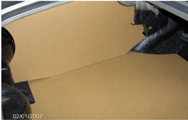
The left panel is the first one in place. The rear cutout should be pulled back enough to fit against the tail light housing.
