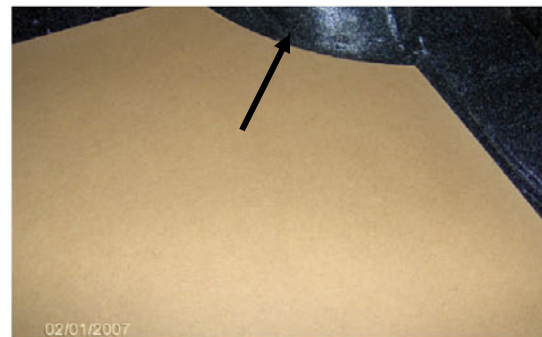
The corners fit around wheel well with enough room for carpeting.
