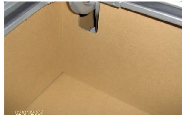
The panels will be snug once the upholstery and carpeting is put into place. You may need to sand them down if using thick material.
