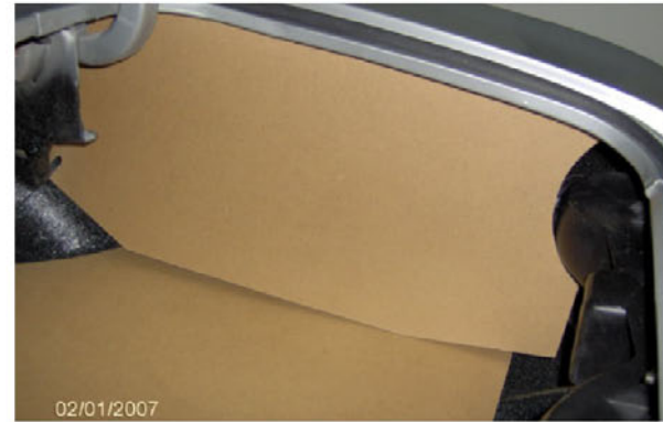
The right panel is next and should also be against the tail light housing.
