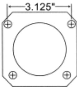
This kit is for axle with a 3 1/8" spread center to center on the top two bolt holes (pictured left). If your axle flange measures 3 3/8" from center to center, you need our kit FSCRD01.
