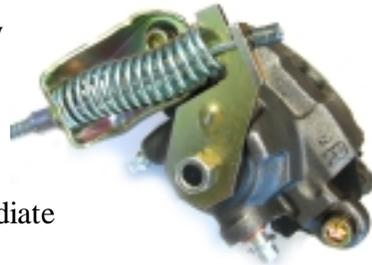
After the cables are installed, you need to adjust the system. Engage and release the emergency brake lever several times to activate the self-adjustment mechanism built into the calipers. You'll know you've got it when emergency brake is fully engaged and the rear wheels will no longer turn by hand.
