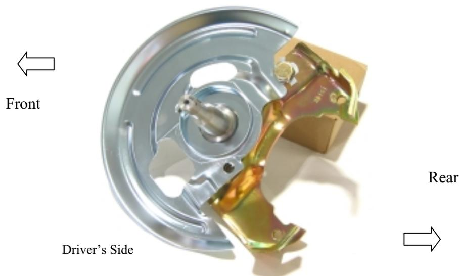
Reinstall your old steering arm with the new bolts supplied with your kit. Place the tie rod end back into the steering arm and fasten it with the original castle nut. Torque the nut to the specifications provided in the assembly manual. Fix it in place with the new cotter pin supplied with your kit. Now is a good time to reattach the sway bar link if you removed it earlier.
