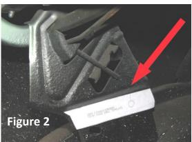
with the supplied stainless steel button head bolts and aluminum washers. Realign the trunk lid on the car as necessary using your markings as a guide and securely tighten the fasteners.
