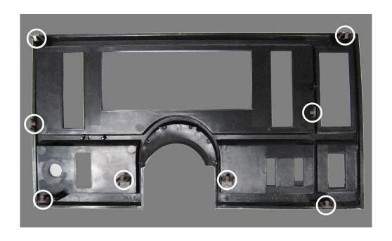
2. Remove the stock gauges by removing the four screws securing the gauges to the dash. A 7mm nut driver will work best for these screws. Keep the screws because they will be used to install the VHX gauges.
