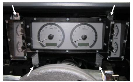
4b. Align the four mounting holes and re-use the factory screws to fasten the VHX gauges into the dash.
