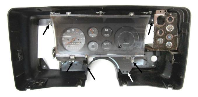
3. Remove the factory gauges by removing the screws shown in the picture below. Your cluster may vary depending on the factory equipment.
