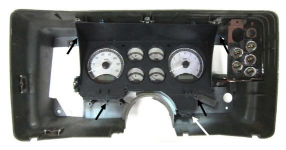
8. If the instrument housing was removed from the dashboard, reinstall, then attach the bezel to the housing with the seven factory screws removed in Step One. Refer to the main manual for wiring instructions to
