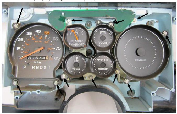
4. You should be left with a bare housing. Remove all light bulbs and electrical contacts, as they are not needed for the VHX system.
