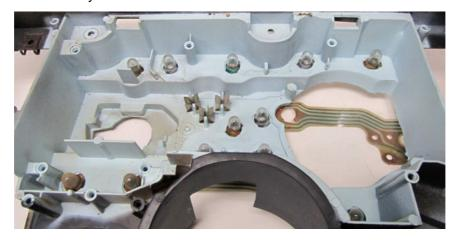
5. Using a die grinder, Dremel tool, or cut-off wheel, carefully trim the plastic bosses as shown. This is necessary to mount the new gauge system.
