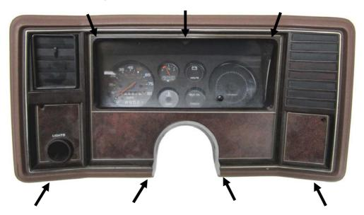
2. Remove the six screws securing the blackout plate and lens to expose the factory gauges. These screws will be reused.
