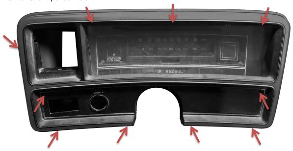
2. Remove the factory lens and faceplate by removing the screws shown in the picture below. Your cluster may vary depending on the factory options installed. Retain these screws for securing the VHX system.
