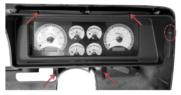
6. If the instrument housing was removed from the dashboard, reinstall, then attach the bezel to the housing with the ten factory screws removed in Step One.
