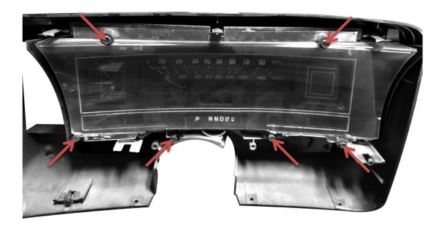
3. Unscrew and remove the factory gauges and plastic light tubes. You should be left with a bare housing. Remove all light bulbs and electrical contacts, as they are not needed for the VHX system.
