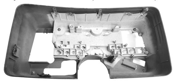
4. Using a die grinder, Dremel tool, or cut-off wheel, carefully trim the plastic bosses as shown. This is necessary to mount the new gauge system.
