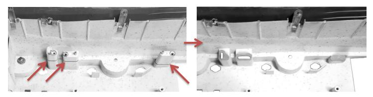
5. With the modifications complete, check fitment and ensure the area circled below clears and doesn't need additional grinding for proper fitment. Connect the CAT5 cable to the display, and feed the cable through the former speedometer cable opening on the rear of the housing. Place the Dakota Digital gauge cluster into the dash, taking care to align the mounting holes with those in the stock dash. Attach the VHX system using the screws retained from step two.
