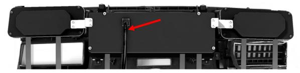
7. Connect the ribbon cables coming out of the main VHX housing to their respective satellite gauges. Each cable is stamped with its corresponding gauge to more easily match them together.
