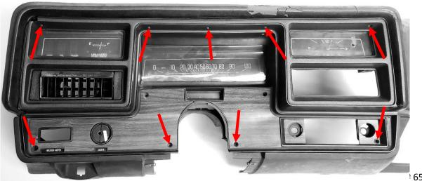
2. Remove the stock gauge cluster from the bezel. The gauge cluster is held in place by four screws in the center of the bezel. Save the screws obtained as they will be re-used to secure the new VHX system.
