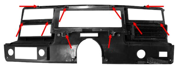
4. Attach left and right satellite gauge pods to main system using the four provided 6-20 x 3/8" screws.
