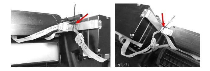
9. When inserting the VHX system and factory bezel into the dash, ensure that the ribbon cables rest in the highlighted locations for the best possible fit:
