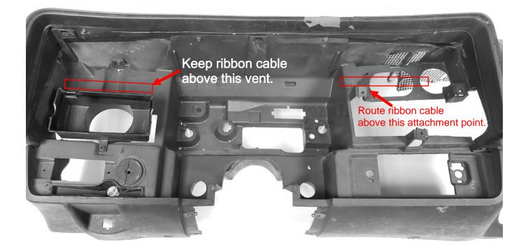
10. Carefully insert the bezel and gauge cluster into the dash, ensuring that the ribbon cables fall into place correctly. Reattach the bezel using the retained original screws.
