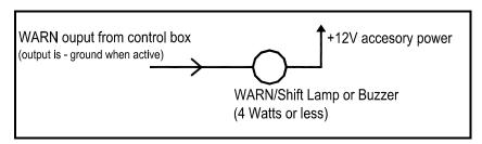
If you need the warn output to be "active high" or provide a +12V voltage to power something larger than 4 watt, a standard 12V relay can be used to accomplish this.
