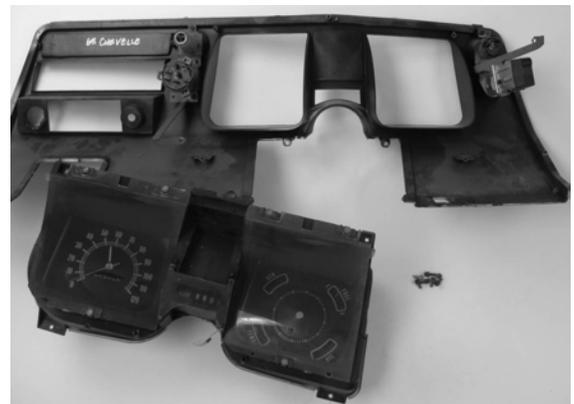
3. Remove the stock gauges from the stock lens spacer. The lens spacer is going to be reused to secure the new VHX gauges to the dash/bezel. Remove seven screws holding the gauges to the spacer. Save the screws, they will be reused to attach the new VHX system.
