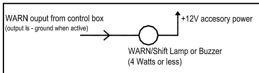
If you need the warn output to be “active high” or provide a +12V voltage to power something larger than 4 watt, a standard 12V relay can be used to accomplish this.
