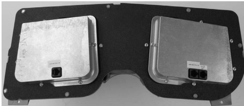
7. Secure the VHX system onto the bezel with the five screws that were removed in step 2.
