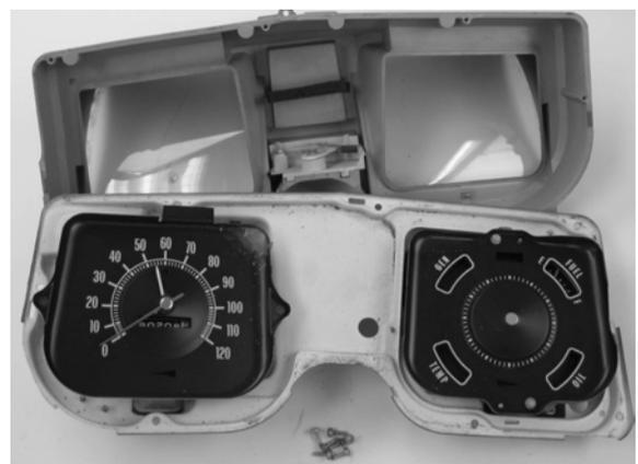
4. Remove the stock lenses from the lens spacer by removing three screws from the front of each lens. The stock lenses are removed since the new VHX kit features a hard coated clear lens. Now is a good time to clean the stock lens spacer as it is reused to secure and space the new VHX system.
