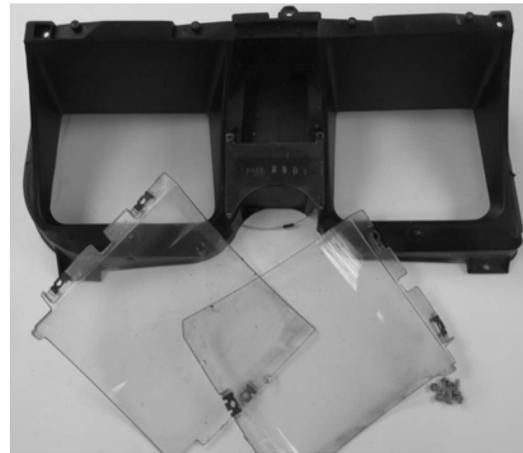
5. This step is optional for automatic transmission bezels only. If you purchased a separate GSS-2000 kit from Dakota Digital, the gear position can be displayed in the VHX message centers, therefore the stock gear position indicator can be removed.
