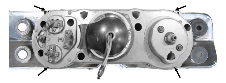
3a. Remove the protective tape from the clear lens and install the VHX system into the bezel.Watch carefully as you insert the system so you don't scratch or damage the lens.
