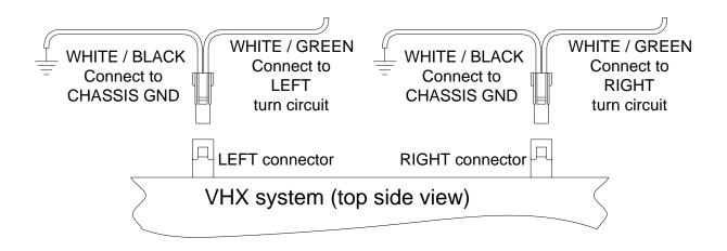
6. Connect the CAT5 cable and the two blinker harnesses to the system. As the assembled cluster is installed into the dash, take care when routing these cables to the control box.
