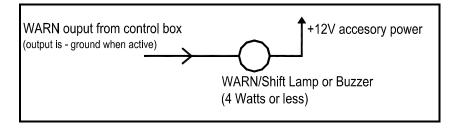
If you need the warn output to be "active high" or provide a +12V voltage to power something larger than 4 watt, a standard 12V relay can be used to accomplish this.
