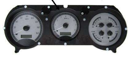
3b. The VHX system should align tightly and the lens should sit flush with the bezel.
