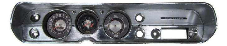
2. Remove the stock gauge, and lens from the bezel. The only items to be reused are the original front bezel and the four screws securing the gauges to the bezel; the other pieces can be discarded. Now is a good time to clean the bezel and remove any dirt or old lens gasket material.
