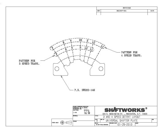
Your Shifter will work for BOTH the 3-speed & 4-speed OverDrive transmissions
