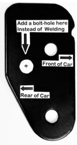
Note: Optional Bolt-hole can be added to rear of plates, as shown above, Instead of Welding! This bolt is needed if Not Welding, to prevent brackets moving when launching hard.
