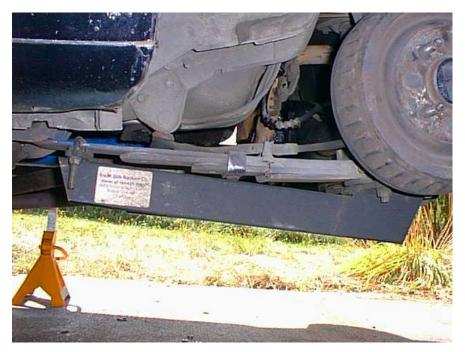
**STEP 12.** If you have a large space between lift bar & leaf springs, you might need to fill this gap with some a small shims, as added below in this application. See Photo Below
