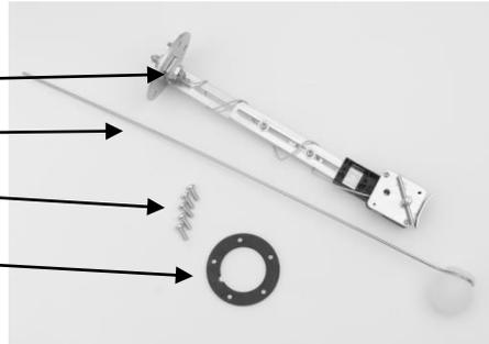
The SEN-06-1 is a 10-180 ohm fuel sender that can be adjusted to work with tanks ranging from 6"-23" deep. The sender has the standard SAE hole pattern and may work for most applications without drilling any additional holes. The steps below will guide you through sender installation and setup. Use care and take necessary precautions when working with a fuel tank that may have or have had some fuel in it. Double check all measurements and mounting spots before drilling or cutting.
