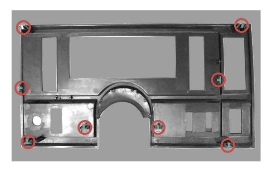
2. Remove the stock gauges by removing the four screws securing the gauges to the dash. A 7mm nut driver will work best for these screws. Keep these screws, as they will be needed to install the RTX system.
