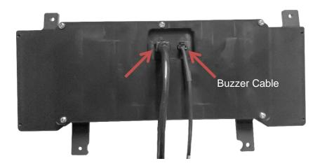
4. Install the RTX system into the dash. Align the four mounting holes and re-use the factory screws to fasten the RTX gauges into the dash.
