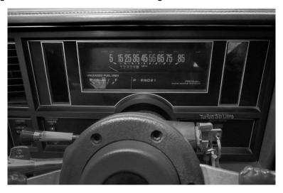
1a. The bezel is held in by push-in clips. Note the locations of the clips on the back side of the bezel. Pull near clips when removing the bezel.
