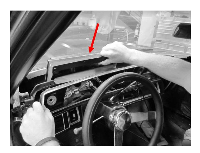
3. Mount the RTX system by sliding the provided screws through the sheet metal dash and plastic dash flange, then thread into the RTX system. Two factory screws will be used to mount the lower portion of the system
