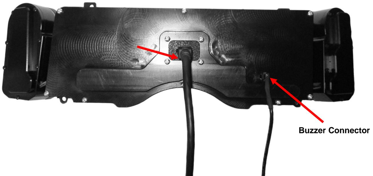
4. Secure the RTX system to the dash with the original four screws.
