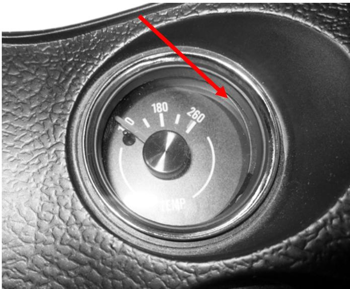
5b. The RTX system should align tightly and the lens should sit flush with the bezel.
