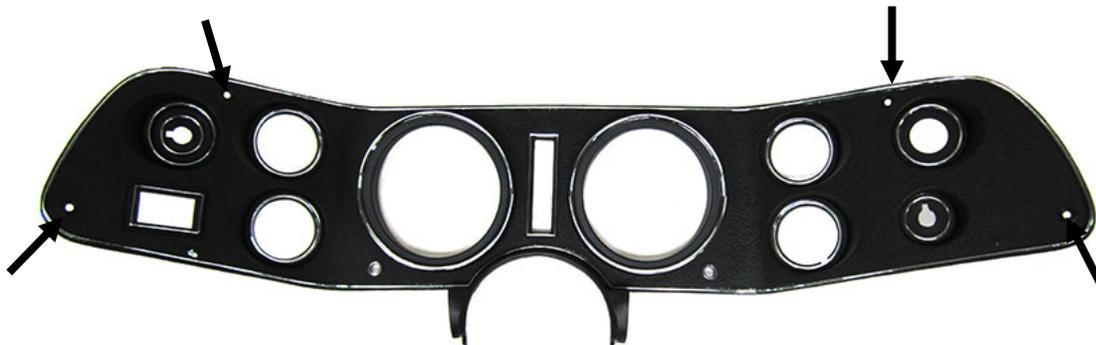
2. Remove the four screws holding the gauges into the dash. These screws will be re-used for the RTX gauge installation.
