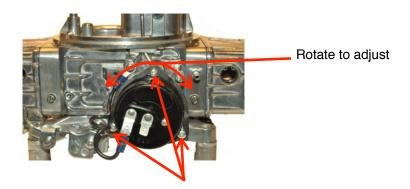
Clockwise rotation reduces temperature for choke to close and shortens the time for the choke plate to completely open. Full clockwise rotation the choke will never close. Counter-clockwise rotation raises the temperature for the choke to close and lengthen the time the choke plate is closed, so it will take longer for the choke plate to open to full vertical position.
