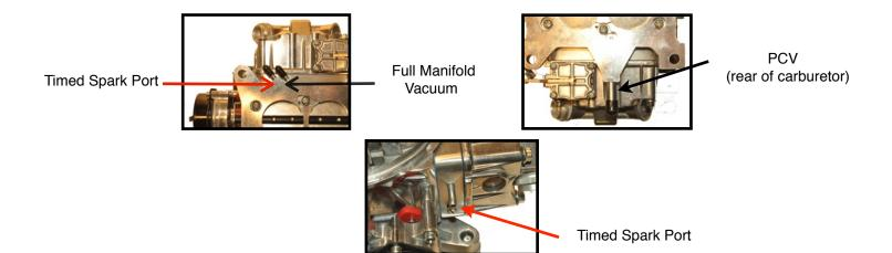
Distributor vacuum advance may also be connected to the tube in the primary metering block.
