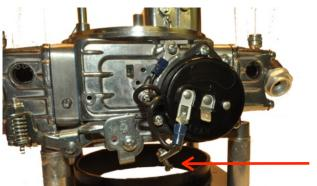
Loosen three retainer screws to adjust choke cap
