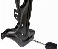
D. With the spoiler now drilled with (3) ¼" holes and the "L" bracket attached to the center, reattach the spoiler using the center mounting point and clamps on each end. You may need to fine-tune the center alignment using the adjustable slots in the "L" bracket.
