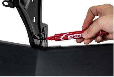
B. While the spoiler is still clamped in place, mark the locations where holes will need to be drilled into the inner bumper brace. We recommend marking these from the underside of the spoiler for best accuracy.
