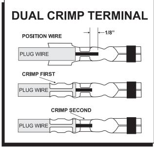
Figure 2 Crimping a Dual Crimp Terminal.
