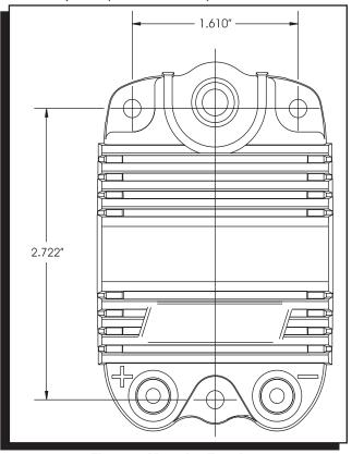
Figure 1 Mounting Template.
