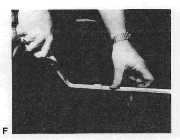
**F.** With pliers, bend end of track to fit inside roof of car.
