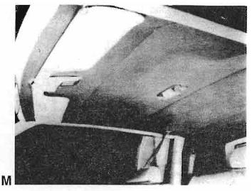
L. Proceed to make a normal headliner installation, cementing above the back window and working forward to the windshield. Cement and trim over door openings so that fabric will be covered by garnish moldings.
