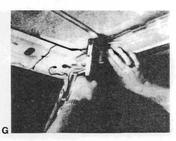
ter as indicated on the drawing included in each kit, pop rivet tracks in place snugly against roof.
