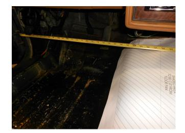
5. Secure the template in place using tape.
