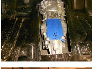
10. Continue drilling all remaining holes. Insert and secure all remaining rivets until tunnel patch is secured to the floor.
