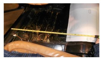
4. Center the front of the template by measuring from the seam located about half way up the forward door jamb to the indicated line on the template.
