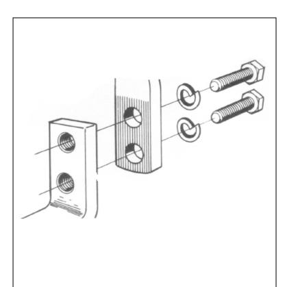
Stick bottom with tapped holes do not require stiffener plate.
