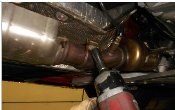
9. Remove the two 15mm nuts from the right side exhaust flange connected to the catalytic converter.
