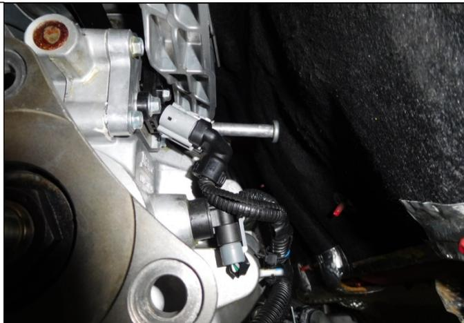
41. Align the link bar with the shift rod on the transmission. Install the supplied linkage pin.
