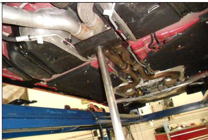
8. Loosen the 15mm nut attaching the left side exhaust flange to the catalytic converter.
