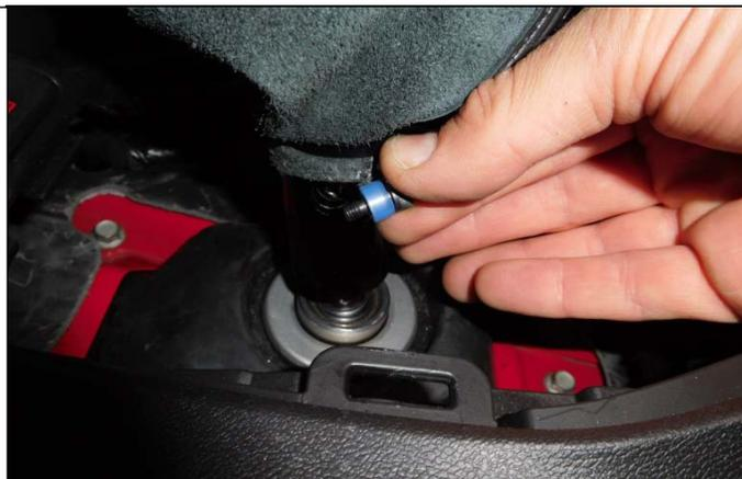
49. Install the shoulder bolts into the pistol grip. Using an 1/8" allen wrench, tighten the shoulder bolts into place.
