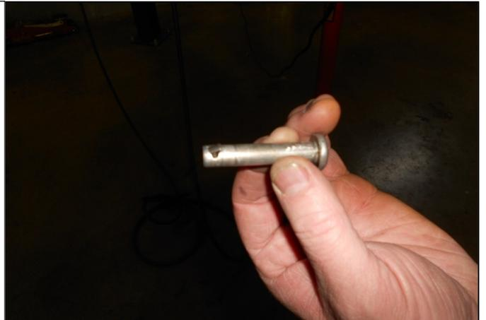
27. Remove the pin on the left and right side by pushing the spring lock down while using a screw driver to pull the pin out until it stops.
