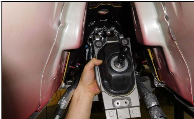
40. Reinstall the two spring pins that attach the shifter housing to the transmission.
