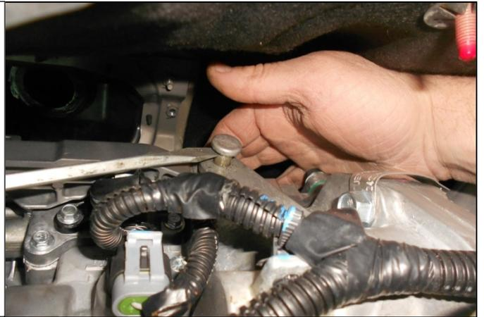
**Note:** The pin can be rolled to gain access to the spring lock.
