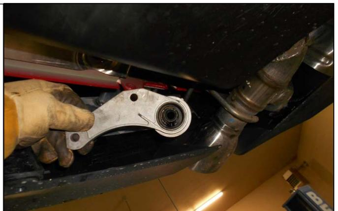
13. The left front exhaust flange is a ball socket you can pry between the transmission cross member and the exhaust to pop it out.
