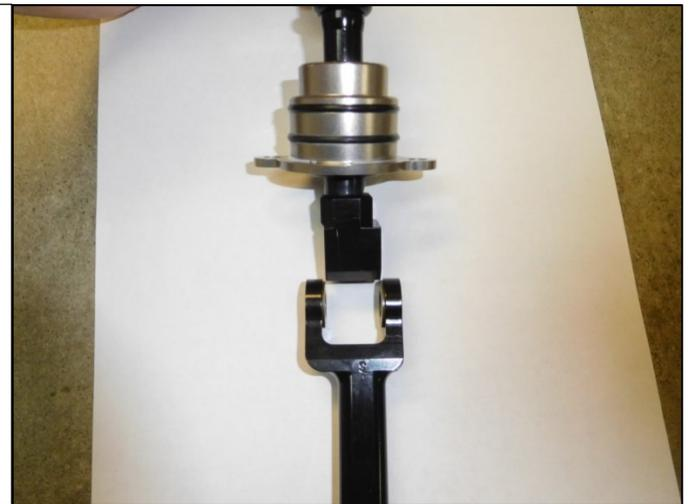
36. Apply grease to the bushings. Insert the supplied linkage pin from the right side of the shifter looking forward. Secure this into place using one of the two factory spring clips that were put aside.
