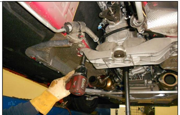
25. Lower the rear of the transmission enough to gain access to the front of the shifter housing.
