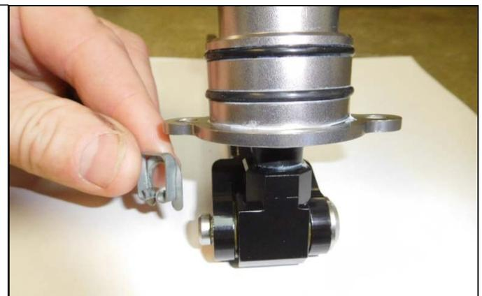
37. Insert the Hurst shifter assembly into the factory housing. Install the supplied bolts. Bolt it in place using a 4mm allen wrench.
