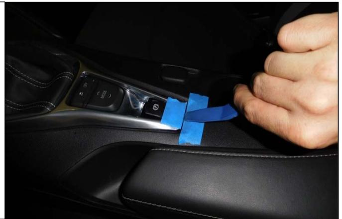
3. Raise the chrome bezel high enough to gain access to the T25 Torx bolt that mounts the shift knob. Remove the bolt.
