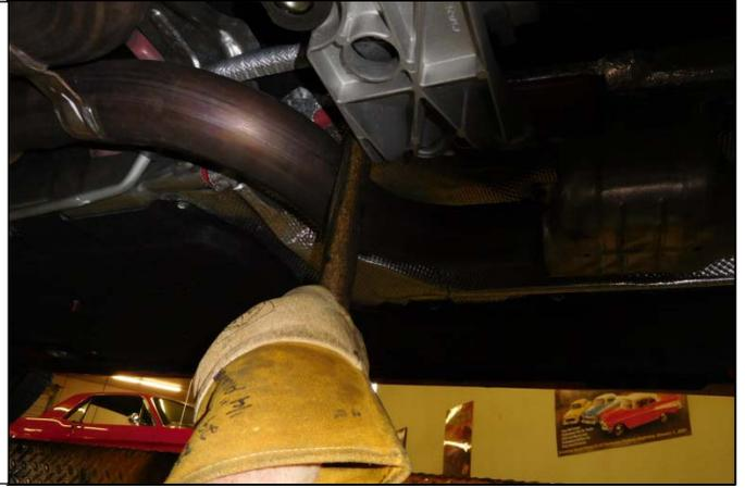
14. Remove the mid hangers on the left and right side of the exhaust. The entire exhaust system can now be removed.
