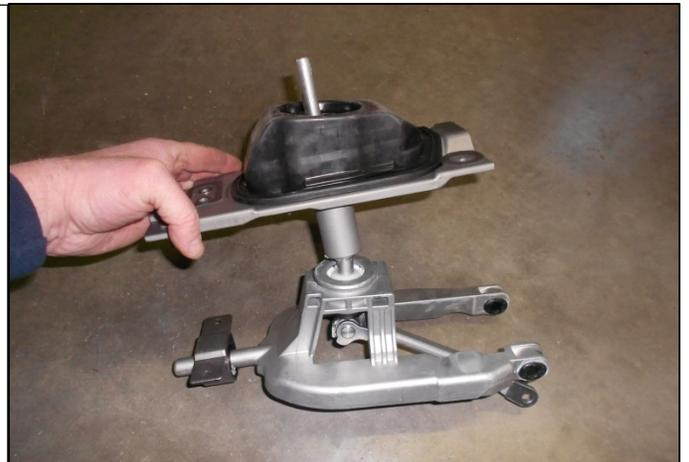
32. Remove the two 4mm allen bolts that hold the factory stick assembly in place.
