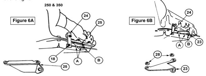
10. Remove the tape from the cable and reinstall one nut and flat washer **B** on the shifter cable. Route the shifter cable through the bracket and reinstall the other flat washer, nut **B**, and two rubber boots **A** (See Figure 2, 6A or 6B).
