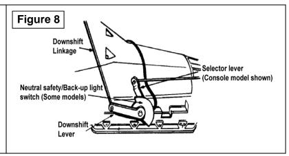
17. The Hurst trans arm must be installed pointing downward. If the factory trans arm C points downward, you must cut off the lower part of the arm at the bend D, to clear the Hurst trans arm (See Figure 9). The Hurst trans arm must be installed so there is an equal amount of travel from center in both directions. Use the ½" x 1 ½" bolt and nut to secure it in place. Make sure the O-ring on the downshift shaft is in position before installing the downshift lever must move freely.
