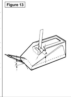
24. Install the console and console cover in position over the shifter mechanism and secure them with two #8 x 1 ¾" and two #8 x ¾" self-tapping screws. Slip the rubber boot over the handle and work it into the console cover. Reinstall the shifter knob.
