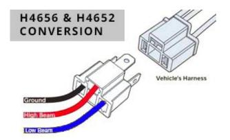
This is the most common wiring scheme of the three terminal 4" x 6" trade numbers (H4652/H4656). This standard has both low and high circuits so be sure to match them up properly.
