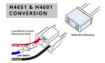
This is the most common wiring scheme of the two terminal 4" x 6" trade numbers (H4651/H5051). This standard has high beam only so insert in whatever manner works best on your application. Confirm the adapter harness wires correspond to the proper wires on the vehicle side when connecting.
