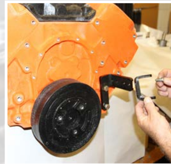
Install pump bracket (2) to L-shaped bracket (1) with bolts (16) and washers (14) supplied
