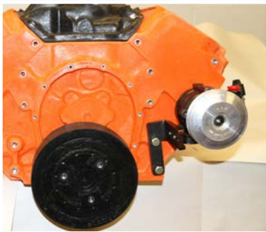
Install pump to bracket (1) using bolts (9) and washers (10) supplied
