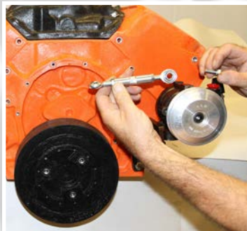
Install adjuster to pump using bolt (9) and washer (10) supplied
