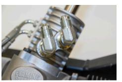
7. If necessary, insert one (1) FR6C6X-S 90° swivel hose fitting into the fitting in the Pressure Port and one (1) FR6C6X-S 90° swivel hose fitting into the fitting in the Return port and tighten. These swivel fittings may only be required to help with issues regarding clearance or fitment.
