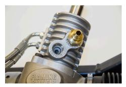
4. In the top Pressure port, insert the FRM14X6AN Pressure fitting and tighten.
