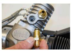
5. Place one (1) 101357 O-Ring onto the FRM16X6AN (M16 X 1.5-AN6) Return fitting.
