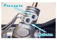
2. Note that each port is labeled Pressure or Return in the rack valve casting.
