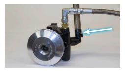
4. Place one end of the 5/8" hose onto the fitting in the Supply port of the power steering pump.
