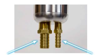
1. Insert the FR125HBL-10-8 (5/8 X 1/2 NPT) barbed hose fitting into the Supply port on the power steering fluid reservoir.
