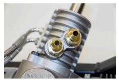
6. In the bottom Return port, insert the FRM16X6AN Return fitting and tighten.
