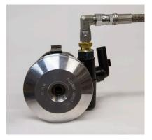
3. If necessary, insert one (1) FR6C6X-S 90° swivel hose fitting into the FRM16X6AN straight fitting on the power steering pump. This swivel fitting may only be required to help with issues regarding clearance or fitment. Then, connect the other end of the hose coming from the Pressure port of the power rack and pinion to the Pressure fitting on the power steering pump.
