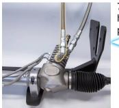
7. Next, attach one end of the 3/8" hose onto the fitting on the Return port of the power rack and pinion.
