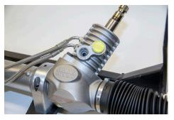
1. Using a pair of pliers, remove the yellow plastic caps covering the Pressure and Return ports on the power rack and pinion.
