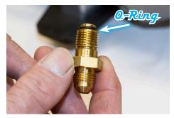
3. Place one (1) 101357 O-Ring onto the FRM14X6AN (M14 X 1.5-AN6) Pressure fitting.
