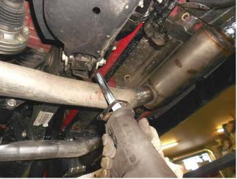
Begin by measuring back  $1\frac{1}{2}$ " from the rear of the suspension cross-member shown in the photos above and make a mark on both pipes. Support the exhaust system both in front and behind the area to be cut, then once you've double checked that the measurements are correct, cut both pipes at the marks. **Note: Use caution when cutting!**
