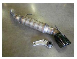
1) Place the new Flowmaster muffler units next to the factory unit and swap the rear hanger mounts from the stock muffler to the Flowmaster assemblies.
