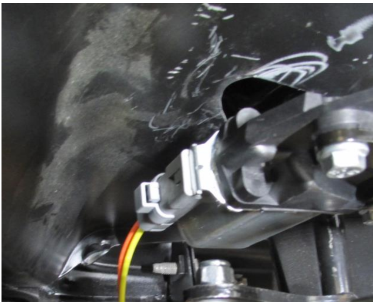
Figure 12 – Connect Harness to Actuators
