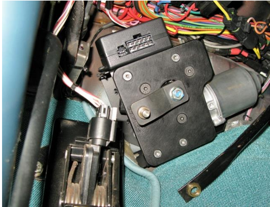
Figure 6 – Install Wiper Motor & Adapter Plate
