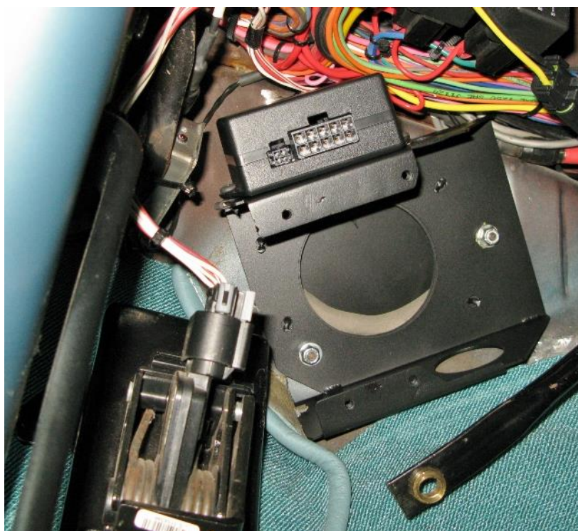
Figure 5 - Install Wiper Control Module
