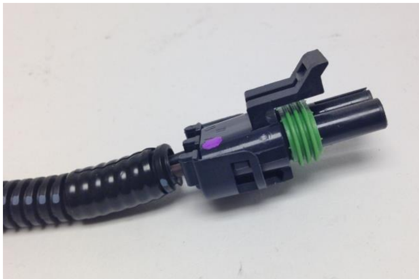
Figure 15 – Washer Pump Connection
