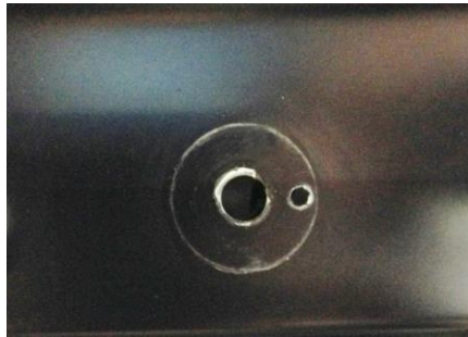
Figure 10 - Drill Anti-Rotation Hole
