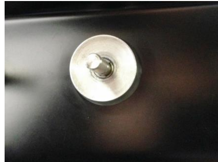
Figure 12 - Thread Bezel onto Switch
