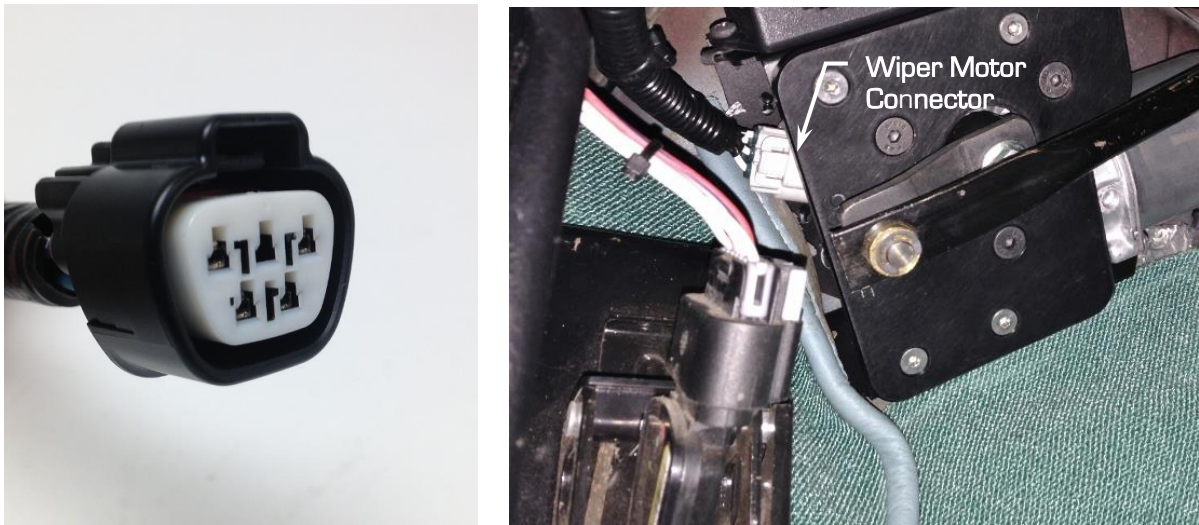
Figure 14 – Wiper Motor Connector
