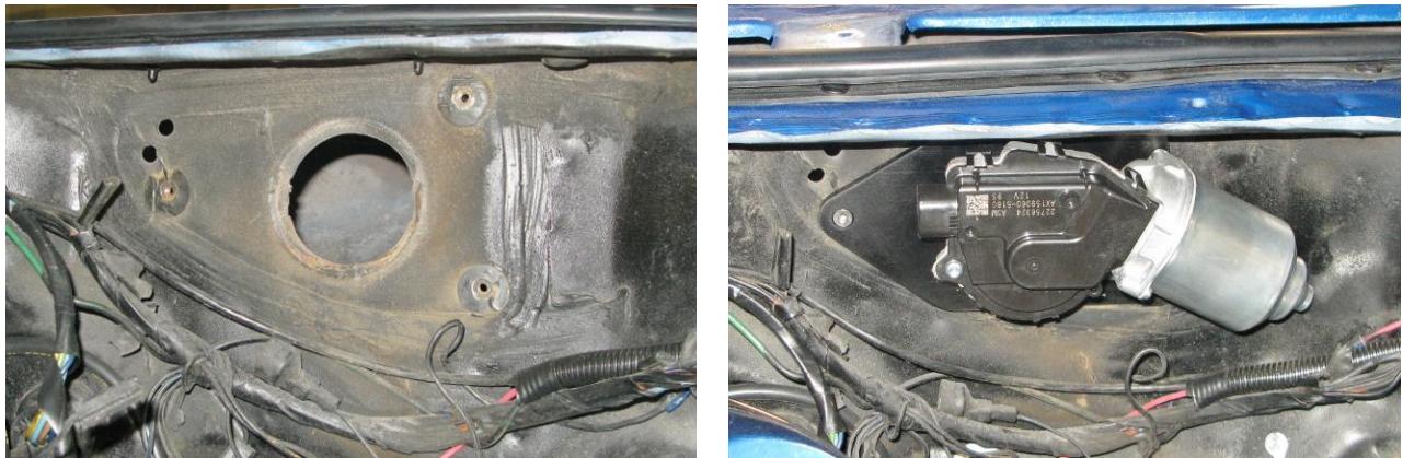
Figure 2 - Wiper Motor Orientation (1970-72 Mounting Plate Shown)
