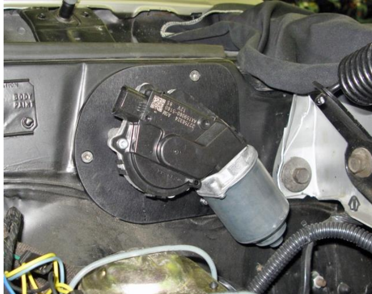
Figure 3 - "Box" Style Wiper Motor
