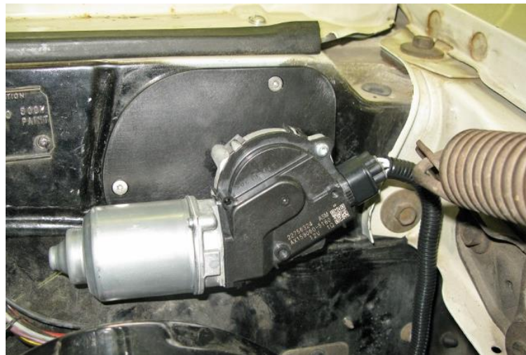
Figure 2 - "Can" Style Wiper Motor
