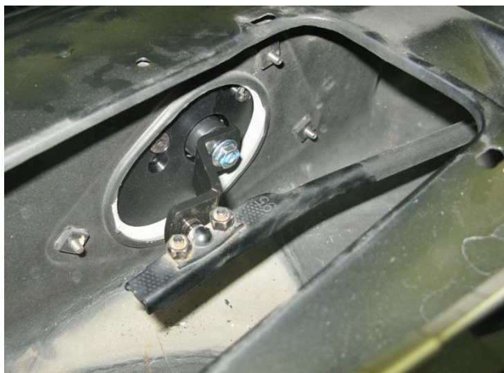
Figure 4 – Attach Pitman Arm to Wiper Linkage
