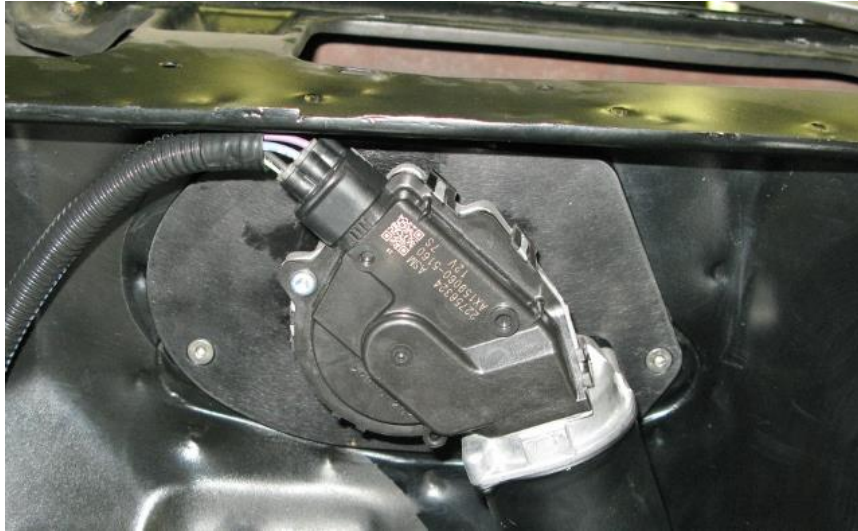
Figure 7 - Install Wiper Motor Connector
