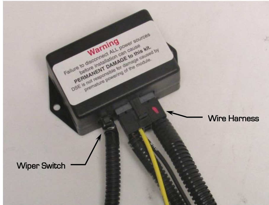
Figure 15 – Connect Wiper Switch & Harness to Module
