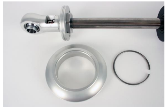
Figure 10 – Spring Seat & Retaining Ring
