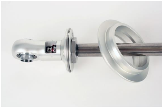
Figure 9 – Remove Upper Spring Seat
