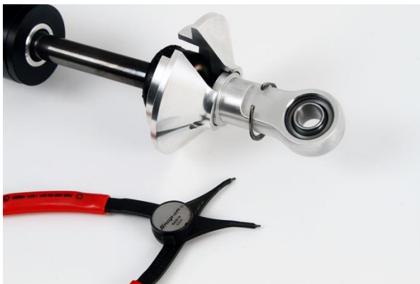
Figure 7 – Removing the Snap Ring
