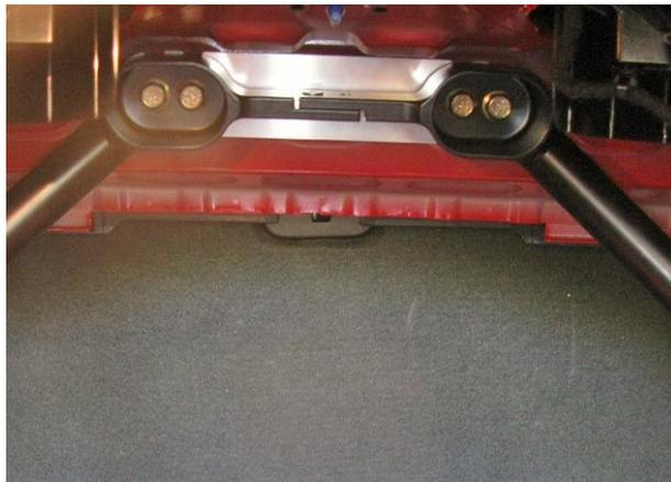
**Figure 14 - Install Upper Shim**
