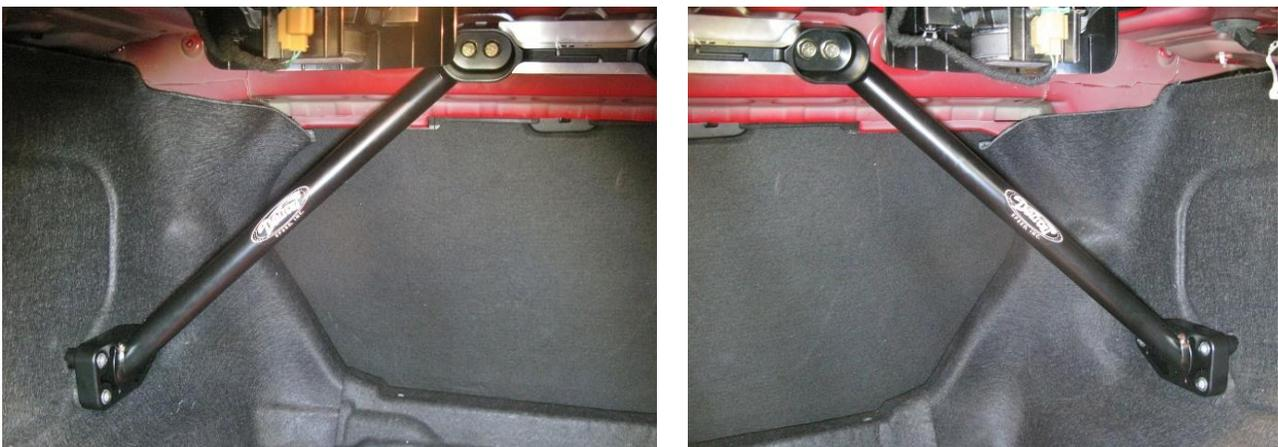
**Figure 15 - Tower Brace Assembly**
