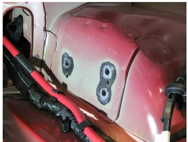
**Figure 4 – Drill-Out Spot Welds**
