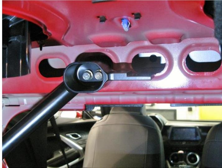
Figure 11 - Attach Upper Mount to Vehicle
