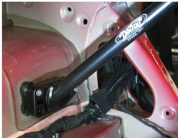
Figure 10 - Position Tower Brace
