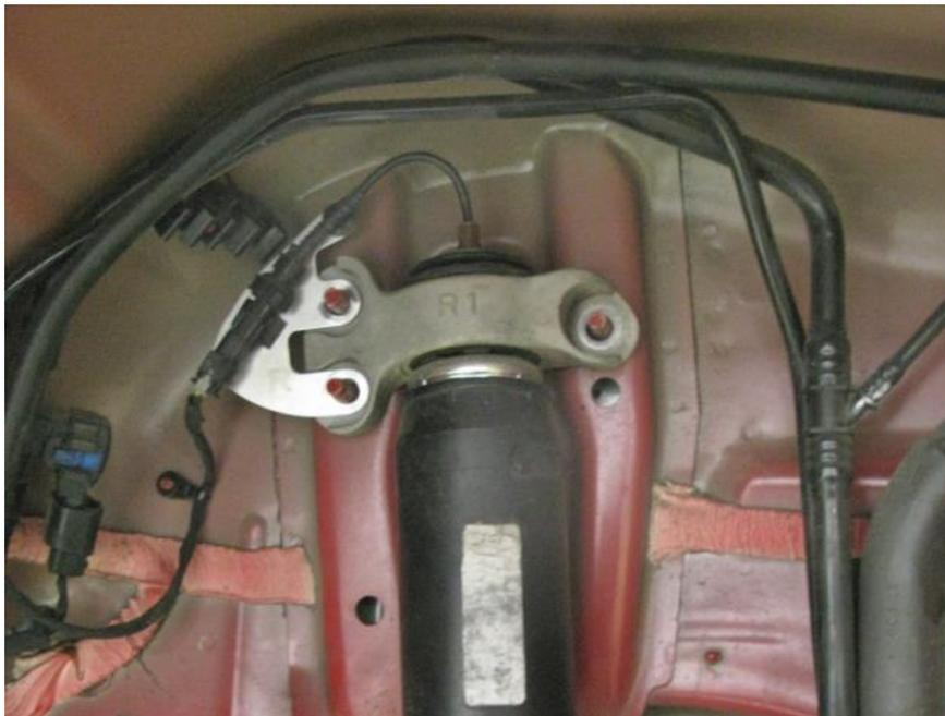
**Figure 6 - Remove Upper Shock Mount Nuts**
