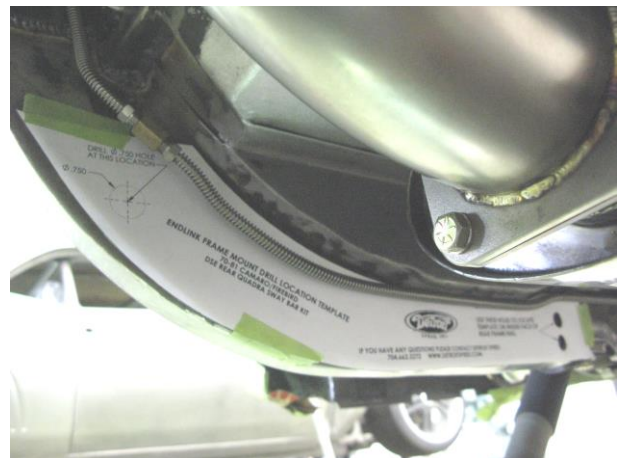
Figure 2 – Positioning the Template on the Framerail
