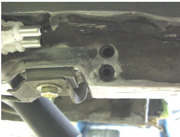
Figure 1 – Locating the Forward Holes in the Framerail
