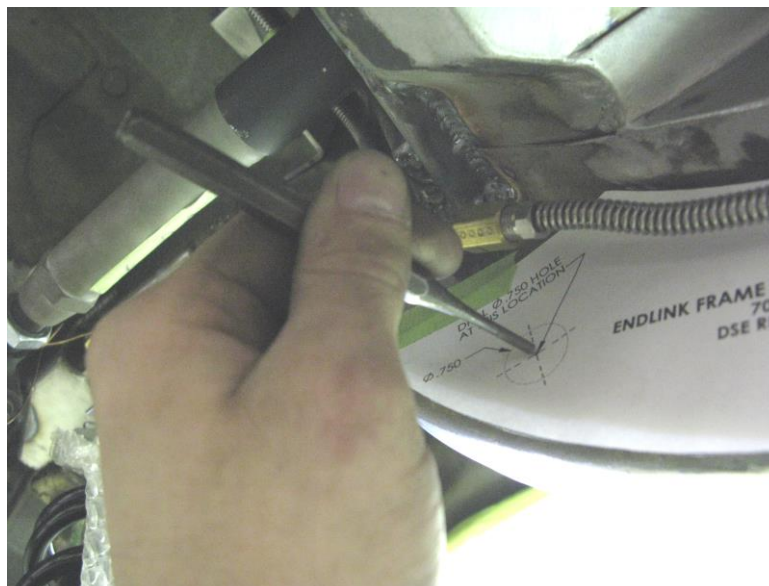
Figure 3 – Locating and Marking the Anti-roll Bar Mounting Hole
