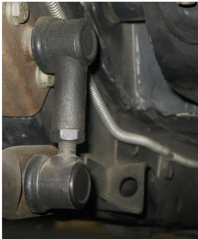
Figure 11 – Anti-Roll Bar End Link
