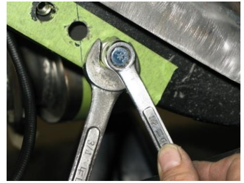
Figure 8 - Installing the Nut Insert
