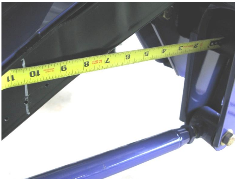
Figure 4 – Measuring for the Anti-roll Bar Mounting Bracket
