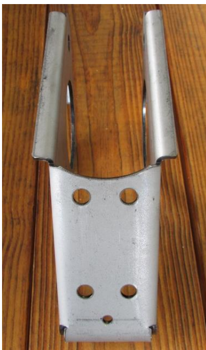
Figure 1 – Pre-Drilled Holes in Coilover Bracket
