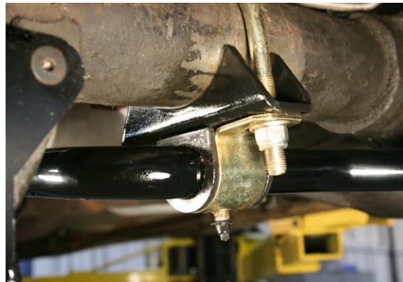
Figure 4 - Anti-Roll Bar Mounted on Rear Axle
