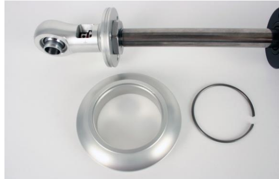
Figure 30 - Spring Seat & Retaining Ring
