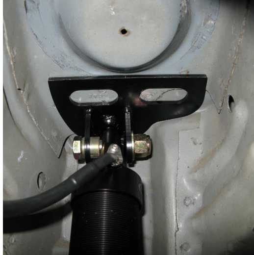
Figure 32 - Remote Canister Shock Shown
