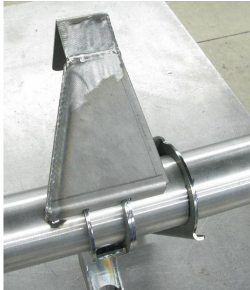
Figure 24 - Track Bar Axle Bracket
