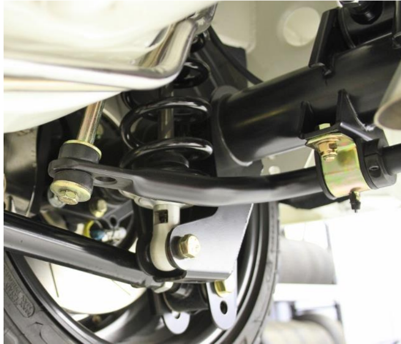
Figure 40 – Install Split Lock Collars
