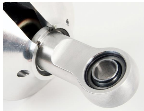
Figure 28 – Snap Ring Installed
