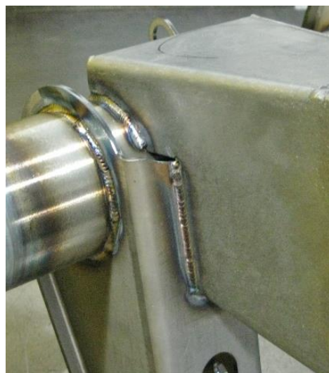
Figure 25 - Finish Weld Track Bar Axle Bracket
