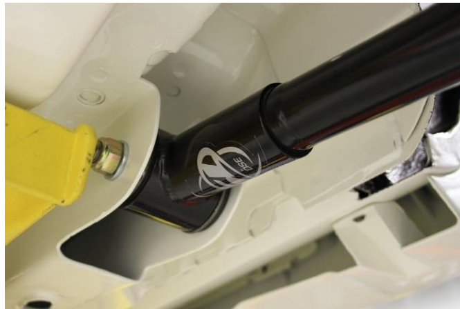
Figure 33 - Lower Swivel Link Body Mount
