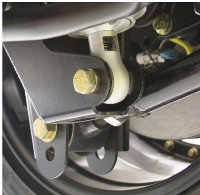
Figure 35 - Shock Adjustment Window
