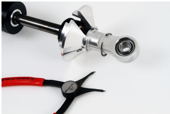
Figure 27 – Removing the Snap Ring
