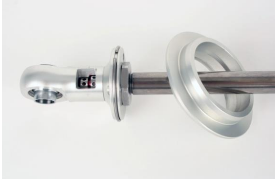
Figure 29 - Remove Upper Spring Seat
