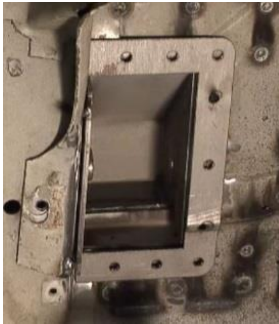
Figure 16 - Plug Weld Close-Out
