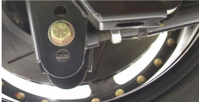
Figure 34 - Lower Swivel Link Axle Mount
