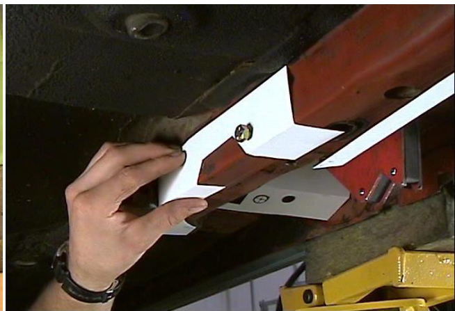
Figure 4 - Leaf Spring Pocket Template - B
