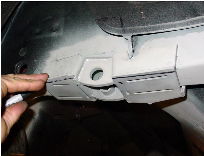
Figure 20 - Trim the Oversized Material
