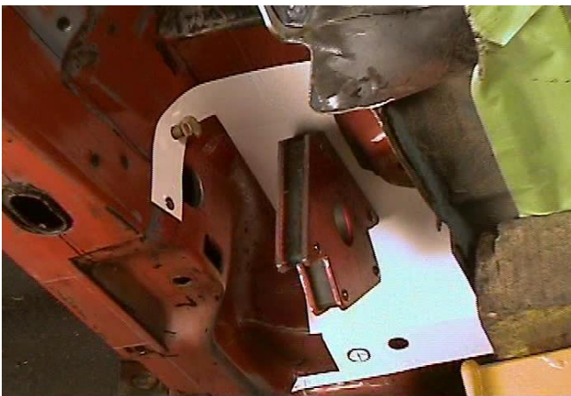
Figure 3 - Leaf Spring Pocket Template - A
