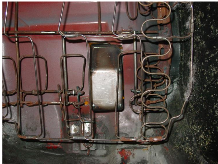
Figure 32 - Modified Seat Frame
