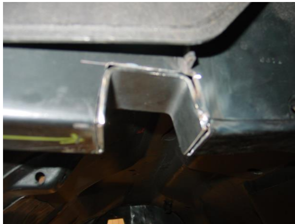
Figure 17 – Frameraill Closeout Tacked in Place
