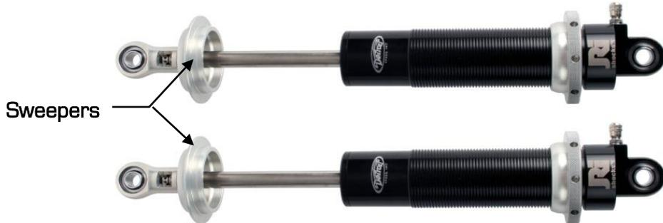
**Figure 19a - Detroit Speed Double Adjustable Shock**
