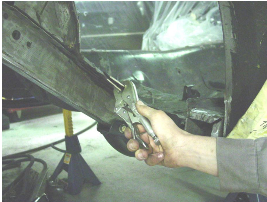
Figure 8 – Folding of Flange
