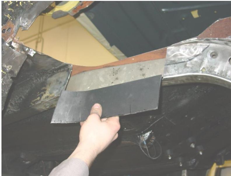
Figure 5 – Frame Rail Closeout
