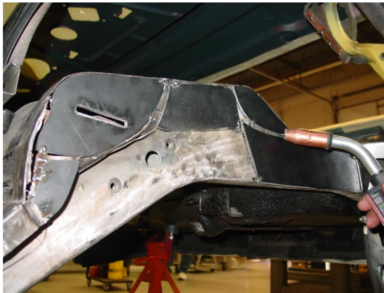
Figure 6 – Mocking up of Templates
