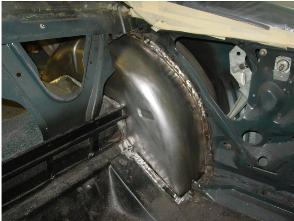
Figure 12 – Welded Tub View (Passenger Compartment)
