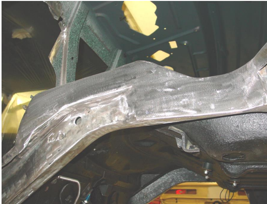
Figure 7 – Framerrail with Closeouts Installed
