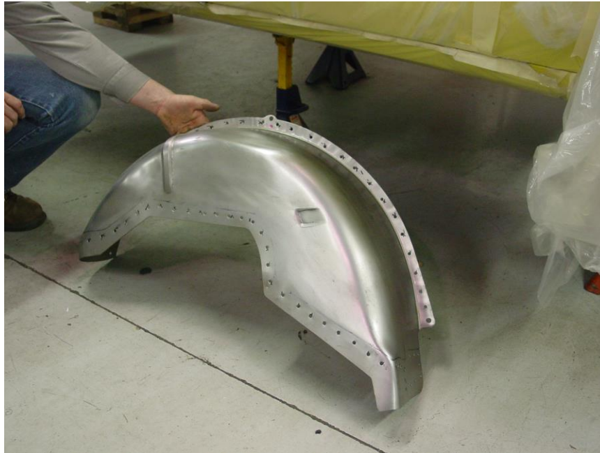
Figure 9 – Tub with Holes Punched
