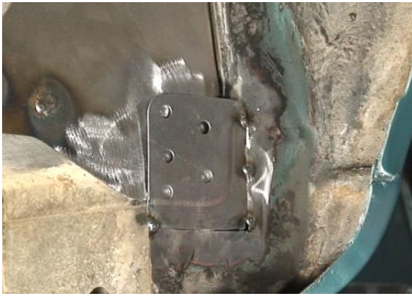
Figure 14a - Welding Fabricated Front Lap Flange
