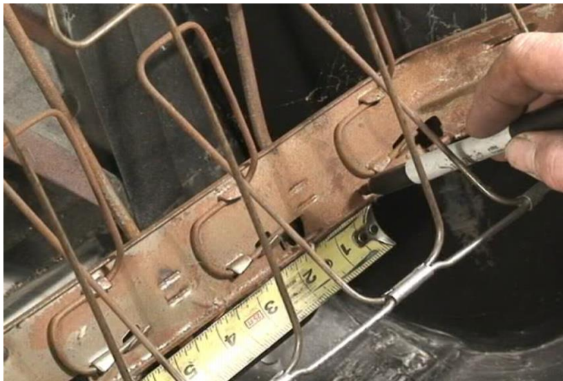
Figure 25 - Cut 2" from Top and Bottom Rail
