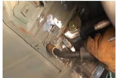
Figure 21c - Welding Anchor [Supported by Anchor Bolt]
