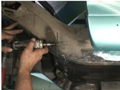
Figure 9a – Mark & Cut Vertical Ends First
