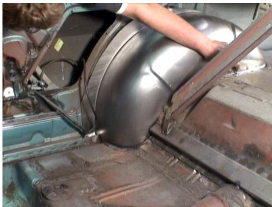
Figure 13a - Marking the Mating Surfaces for Welding
